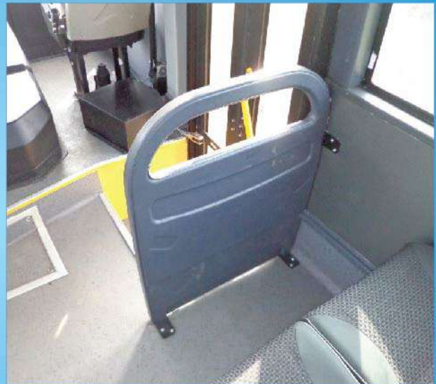
STEP-WELL PARTITION FOR ADDITIONAL SAFETY
